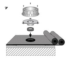
**7** Place the strainer and the strainer cover into the clamping ring of the drain pot.
